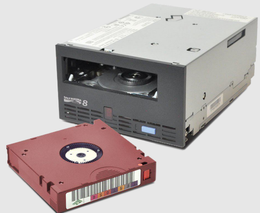
Above: An image of Spectra Logic's LTO-8 tape and tape drive, courtesy of TechTarget .
